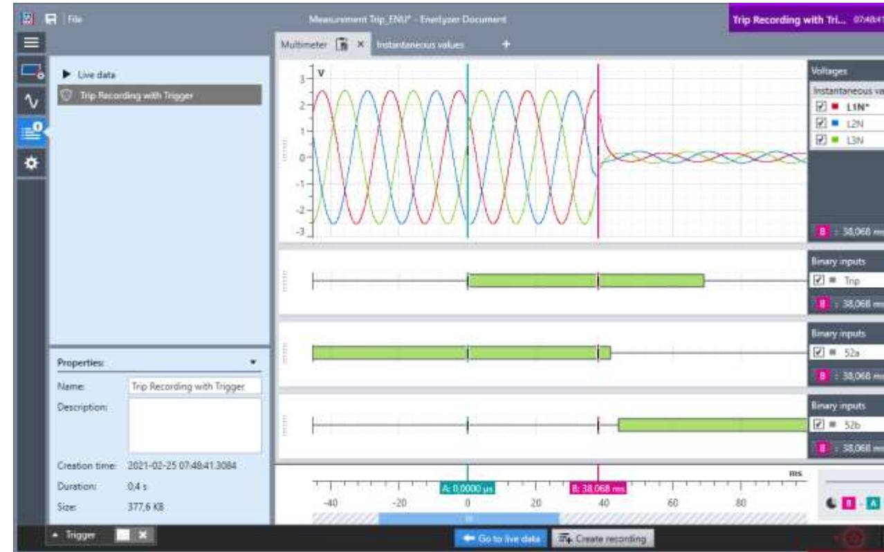
Open-close time measurement of a circuit breaker (optional analog measuring inputs required)
